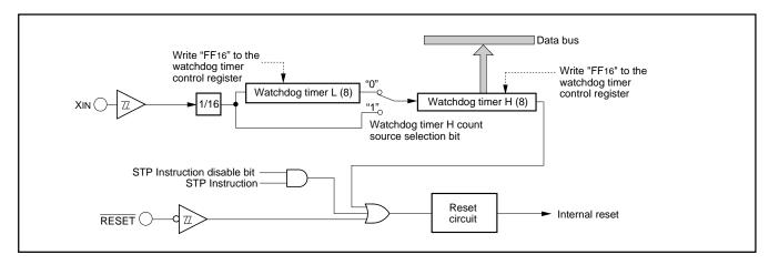
Fig. 41 Block diagram of watchdog timer
