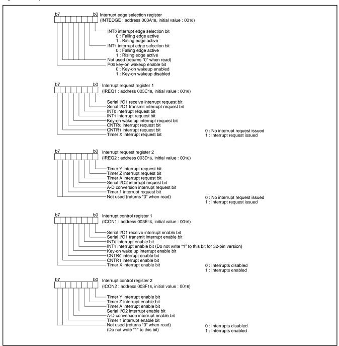
Fig. 20 Structure of Interrupt-related registers
