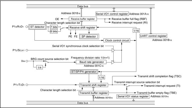
Fig. 32 Block diagram of UART serial I/O1
