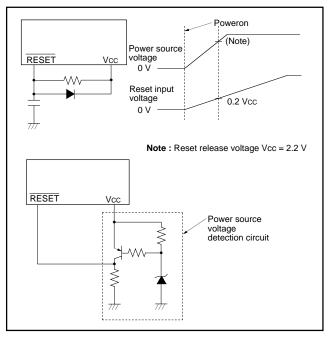
Fig. 43 Example of reset circuit
