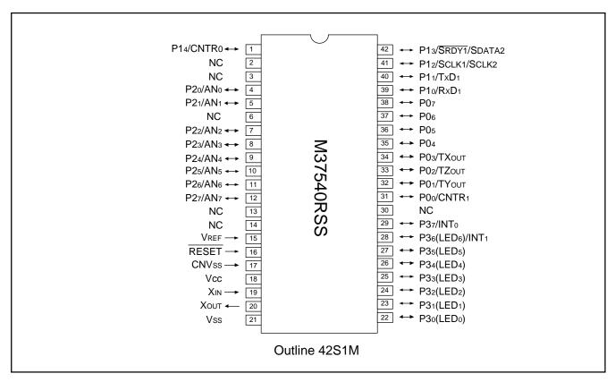
Fig. 4 Pin configuration (42S1M type)
