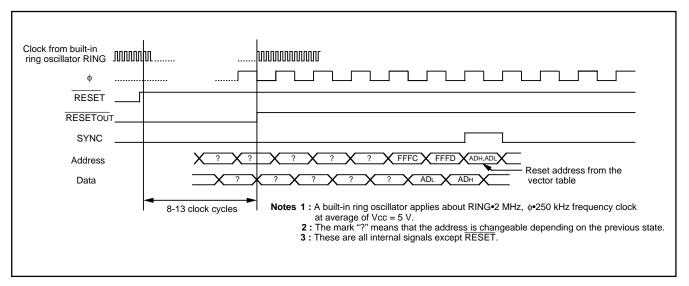
Fig. 44 Timing diagram at reset
