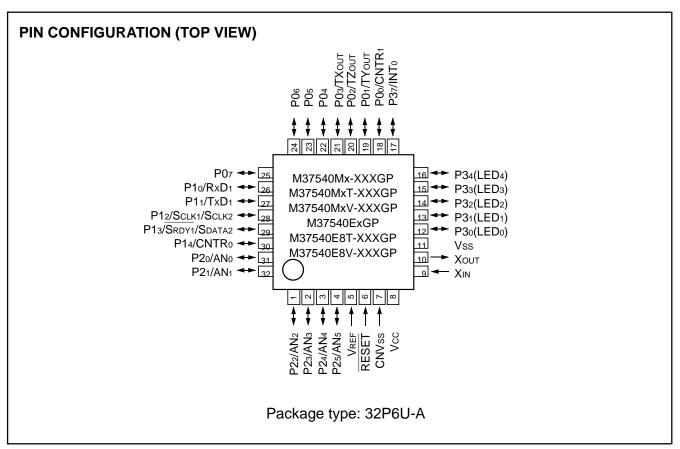
Fig. 1 Pin configuration (32P6U-A type)
