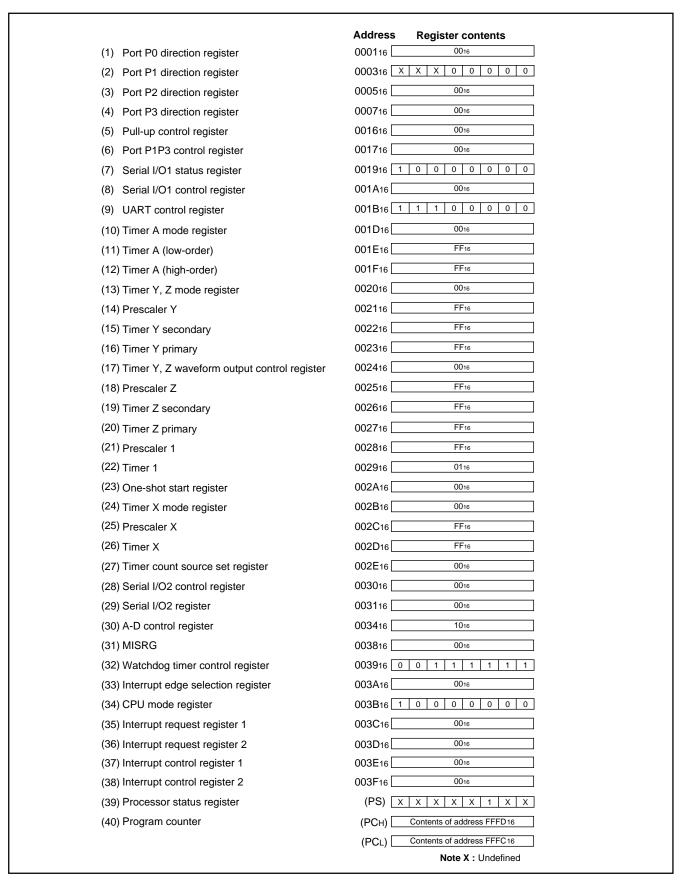
Fig. 45 Internal status of microcomputer at reset
