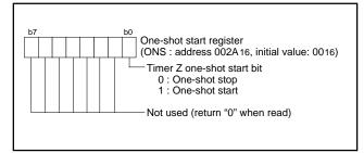
Fig. 27 Structure of one-shot start register
