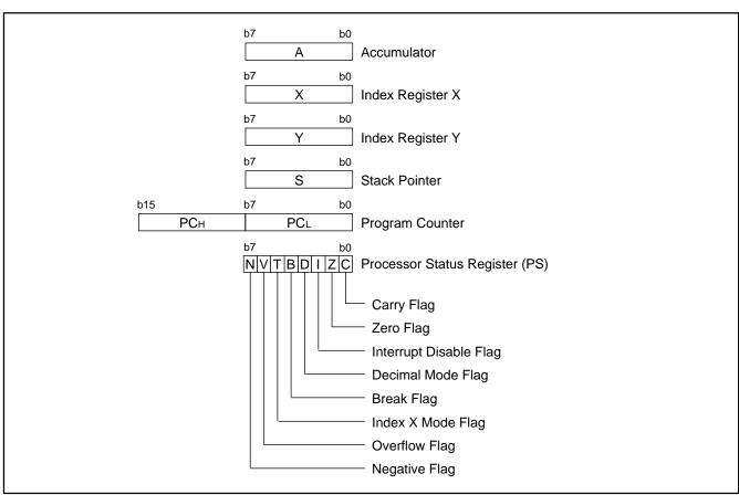
Fig. 9 740 Family CPU register structure
