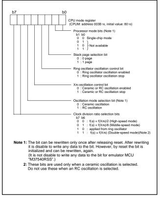
Fig. 11 Structure of CPU mode register
