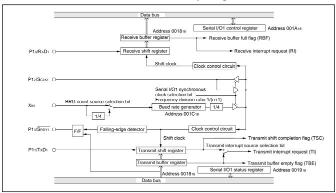
Fig. 30 Block diagram of clock synchronous serial I/O1
