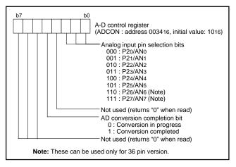
Fig. 38 Structure of A-D control register
