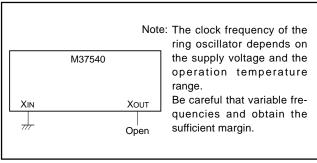
Fig. 49 Processing of XIN and XOUT pins at ring oscillator operation
