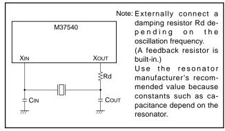
Fig. 46 External circuit of ceramic resonator
