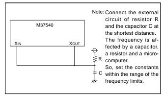
Fig. 47 External circuit of RC oscillation
