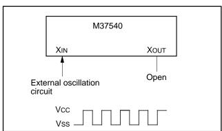
Fig. 48 External clock input circuit
