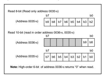
Fig. 39 Structure of A-D conversion register
