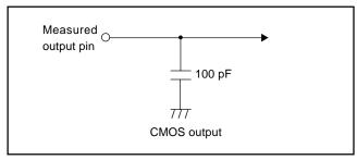
Switching characteristics measurement circuit diagram (General purpose)
