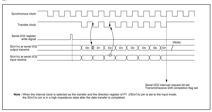
Fig. 37 Serial I/O2 timing (LSB first)
