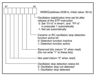
Fig. 50 Structure of MISRG
