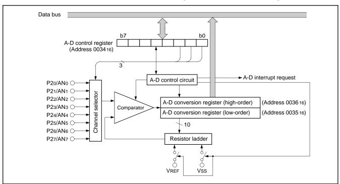
Fig. 40 Block diagram of A-D converter
