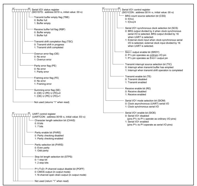
Fig. 34 Structure of serial I/O1-related registers
