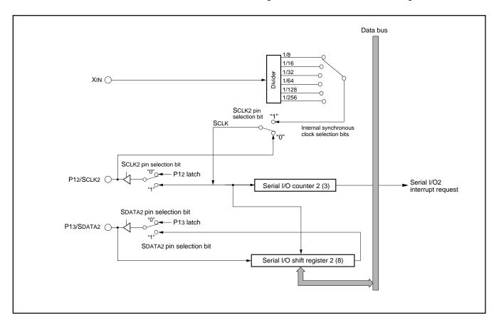
Fig. 36 Block diagram of serial I/O2
