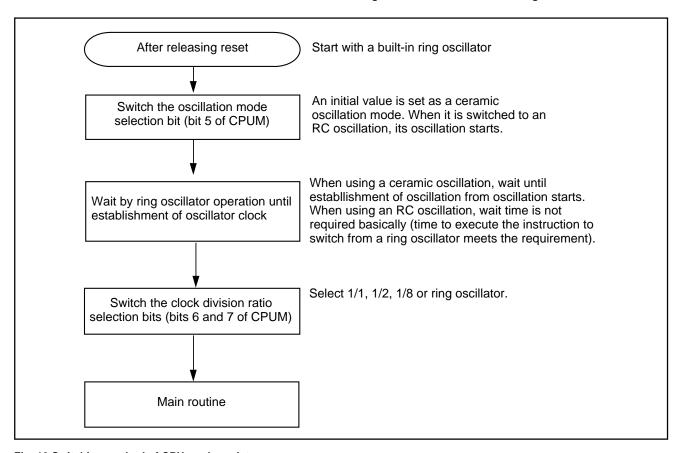
Fig. 12 Switching method of CPU mode register
