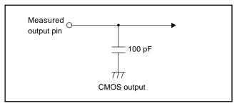
Switching characteristics measurement circuit diagram (General purpose)
