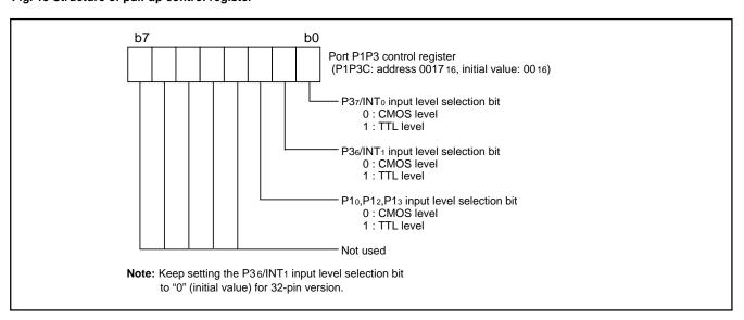
Fig. 16 Structure of port P1P3 control register
