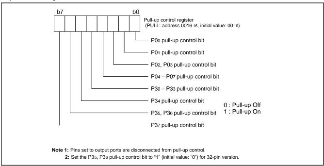
Fig. 15 Structure of pull-up control register
