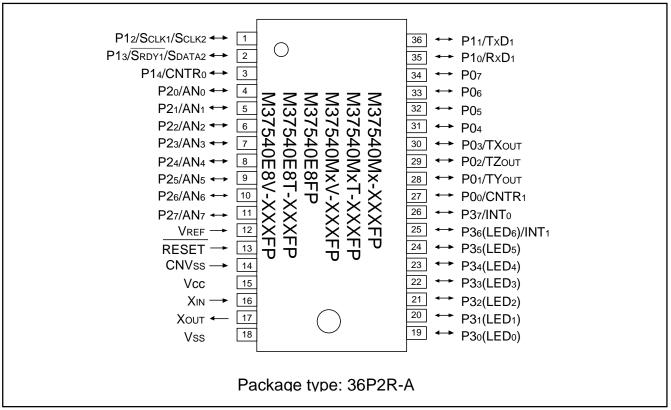
Fig. 2 Pin configuration (36P2R-A type)
