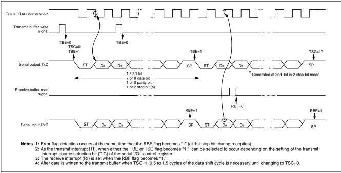
Fig. 33 Operation of UART serial I/O1 function
