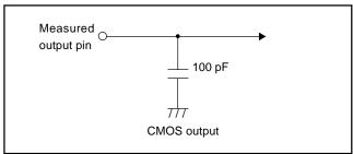
Switching characteristics measurement circuit diagram (General purpose)
