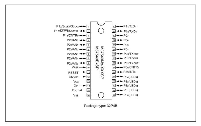
Fig. 3 Pin configuration (32P4B-A type)
